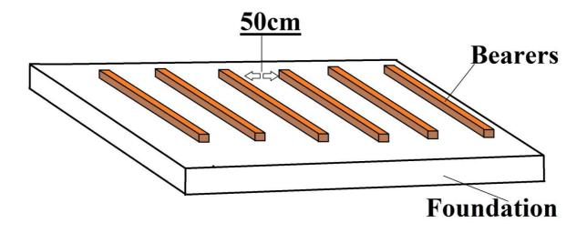
**4.4. Assembling the walls**: place the wall-boards on the bearers as shown in a general sample below (it is not the actual structure plan):
