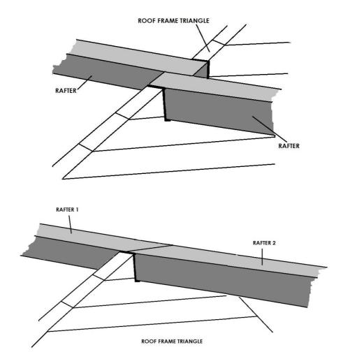
**4.7. Roof-boards:** The next step is to attach the roof-boards vertically and screw them into the rafters. Make sure the ends of the roof-boards are perfectly parallel to each other. Then fix the roof plank boarder under the roof-boards as show below. The roof-plank must be screwed to the roof plank boarder.
