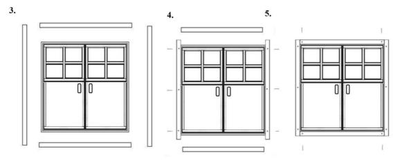
Then insert door frame in to its space from the outside of the structure and attach the rest of the support trims.
